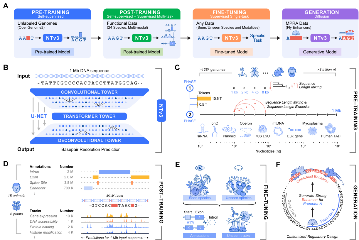
Figure 1 | Overview of model architecture, training procedure and applications for NTv3. A) Different phases of NTv3 training and applications. B) Core U-Net-style architecture for 1 Mb, single-bp modeling, comprising convolutional downsampling, a long-range Transformer core, and deconvolutional upsampling. C) Multispecies post-training on functional tracks and genome annotations across 24 species using a joint objective that combines supervised track and annotation prediction with continued MLM. D) We introduce a new NTv3 BENCHMARK and evaluate various models through fine-tuning. E) Generative extension in which NTv3 is adapted via masked diffusion to enable controllable enhancer design with promoter-specific activity.
